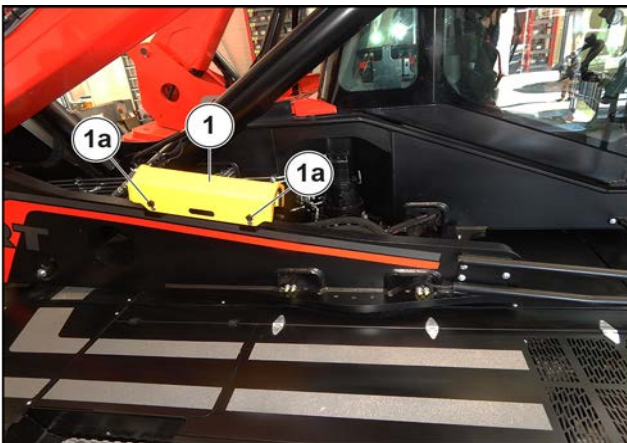
Figure 67: Boom safety wedge
