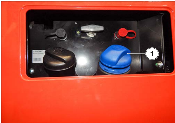
Figure 122: Filling the "DEF" tank
